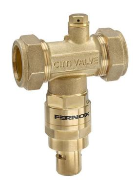
The Fernox TF1 Antifreeze Valve is specifically designed to protect water-based air and ground source Heat Pump heating systems. In cold weather when temperatures drop, systems that are not treated with a glycol-based fluid can freeze within the heat pump circuit potentially causing harmful and costly damage to vulnerable heat pump components and system pipework; eventually causing premature breakdown and repair.
