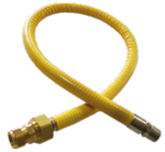
Kitemarked approved by BSI. Manufactured and approved to European Standard EN15266 : 2007, referring to 'Stainless Steel pilable corrugated tubing kits in buildings for gas with an operating pressure upto 0.5bar'. This hose can not be fitted to moveable/free standing cookers. Suitable for both natural gas and LPG. Can be cut to length if required
