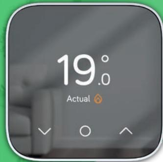
**Modulation:** Traditional thermostats work by turning the boiler on when the temperature reaches a pre-set minimum temperature, and turns off when that temperature is reached. Heat pumps are most efficient when they maintain a steady temperature, so the thermostat modulates the output to keep a constant temperature.
